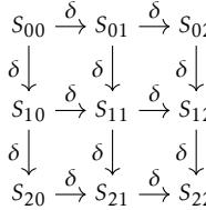
In this example, the inner loop is not vectorisable since there is a dependence chain linking successive iterations. Similarly, outer loop is not parallel. This loop nest has two dependence distance vecs,  $(1, 0)$  by outer loop and  $(0, 1)$  by inner loop.
