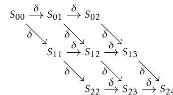
Now we can interchange for **top down lexicographic traversal** (i.e.  $S_{00}, S_{01}, S_{11}, S_{02}, S_{12}, S_{22}, \dots$ ). Now, iterations in each column are independent, so the inner loop is vectorisable.
